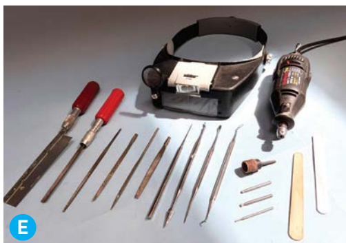
Foam sculpting tools: modeler's saw, hand files, dental picks, Dremel with bits, emery boards, and magnifier
